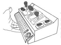
To apply legends for the function keys, pry up carefully, but with force, on the panel cover, place the legend strips above the keys. Insert the top of the panel cover first, and snap the bottom back into place.
