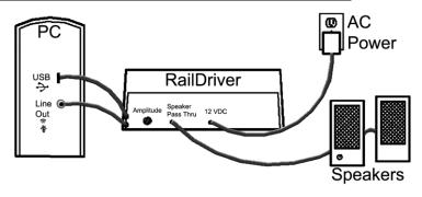
The following steps are required to enable the RailDriver internal subwoofer. Power and audio connections are not required for operation of the RailDriver controls, but they do enhance the driving experience.
